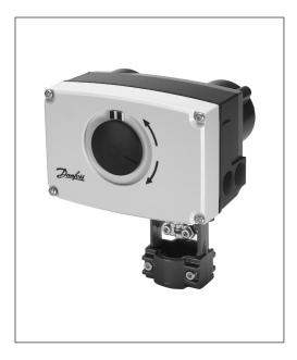
AME 25 SD or SU electric actuators are used with valves gen.2009 type VRB, VRG, VF, VL with additional adapter (Code No. 065Z0311, not supplied) and VFS 2 valves up to DN 50 diameter. The actuator automatically adapts its stroke to valve end positions which reduces commissioning time.
