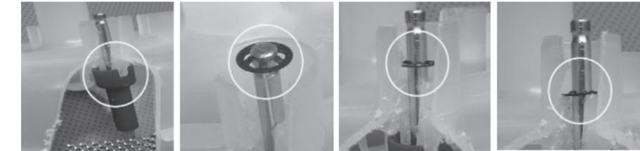
1. Insert the electrodes on the cover until the plastic supports are up against the corresponding notches.
