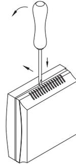
To open the enclosure, set a screwdriver (2.0) in the groove at centre, press down, and lift up the bottom frame slightly. Pull top cover forward and hold it.
