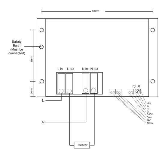
NOTE: It is imperative that the power connections are fully tightened, without excessive force, and ensure the maximum area of cable is in contact with the terminals.
